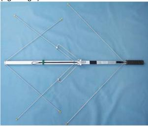
3. Loosen the screws on the center balun just enough to allow the small T-Match rods to be inserted freely. DO NOT loosen the lug screws that hold the T-Match rods to the driven element. These two lug screws should never be loosened, and should be tightened if they become loose.
