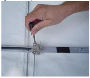
4. Open up the center two element rods carefully, and insert the T-Match rods into the balun holes until the elements are set at 90 degrees or at right angles to the center mast.
